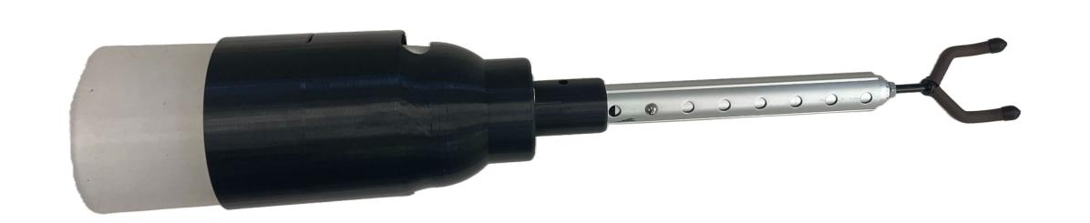
Prototype achieves core functions: adjustable forearm and upper arm, quick release with prong hand attachment, and stable component design. We were unable to find volunteers with above elbow limb differences. Future work should include:
